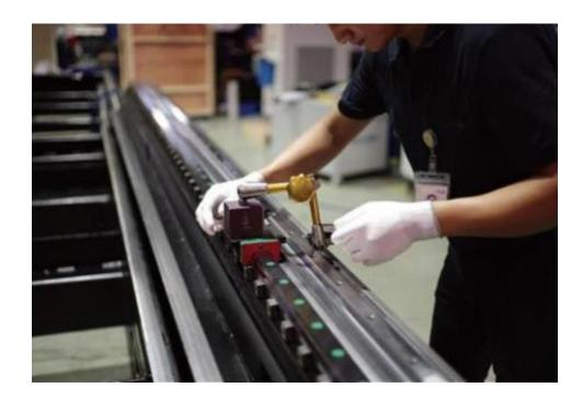
• A collimator is run along the fulllength of the guide rail, testing for straightness. Adjustments are made as required to ensure linear accurate linear accuracy.
