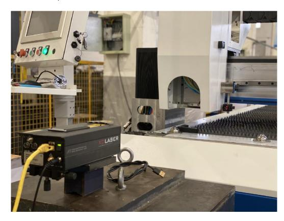
•A Marble test is performed to measure theXand Y axis, calculating any necessary adjustments to ensure perfect level and alignment along length of machine.
